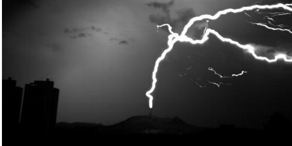
Figure 7 - Time-integrated video segment from the high-speed camera (4.000 ips, 250 \mu s exposure) showing the development of bright RLs on the weakly luminous branches. Many of the RLs faded prior to connecting to a main channel.
